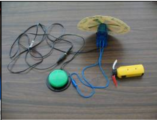
Dollar Store fan converted into a portable spinner and used with a battery interrupter
