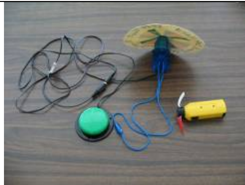
Dollar Store fan converted into a portable spinner and used with a battery interrupter
