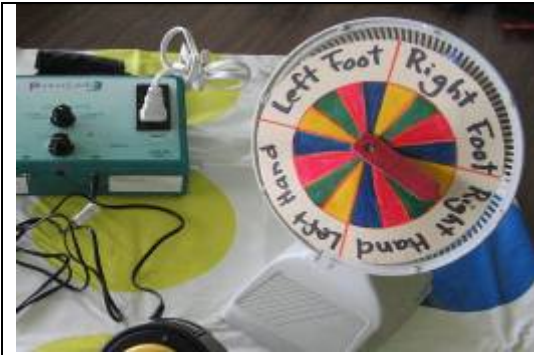
Any fan can be converted into a spinner, when plugged into the Powerlink with a switch.
